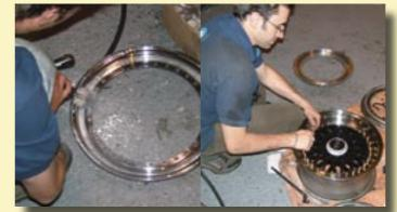
11 The Storm Developments crew supplied the bolts and got busy polishing the half inch outers for the front wheels. Ensure the holes line up before Loctite-ing and torquing the bolts to 10ft.lb
