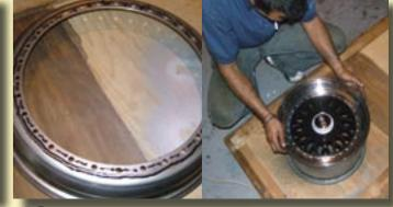
10 Flip the outer over and place some sealant between each bolt hole and around the outer edge. Any excess will squeeze through the holes when you tighten the bolts, rub it off ASAP
