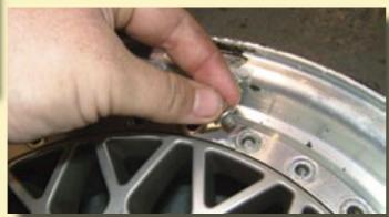
13 ...just like this. Be particularly careful if you take the 'lazy' route and use an air gun to undo the bolts. If you strip the internal thread of the wheel then it could prove expensive
