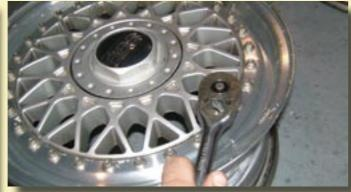
**02** An 8mm splined socket and ratchet will loosen the 30 bolts that hold each wheel together. Try not to exert too much pressure on them as they're prone to snapping in the rim...
