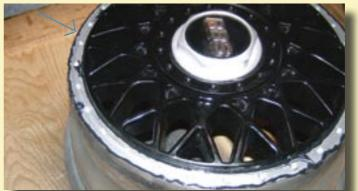
**09** Then switch to the outside edge of the wheel centre. A thin bead here will squeeze up between the outer and inner to form an airtight seal.
