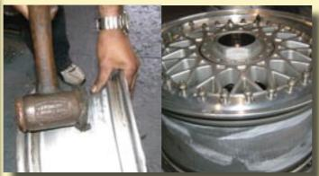
Place a soft cloth on the floor to catch the precious lip, assuming yours are good enough to keep, polish up and sell on. Use a rubber mallet to shock the outer rim and free it.
